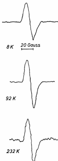
Fig. 3. Examples of the first derivative of the proton NMR absorption spectra of 2-methyl-piperazine obtained at 10 MHz and various temperatures.
